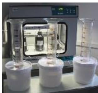
Photo 1. Gas measuring system for microfermentation
